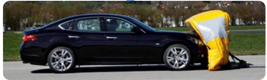
Testing an emergency braking assistant. Source: ADAC e.V.
